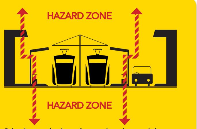
Below the ground and up to 3 metres above the ground, the hazard zone extends 2 metres either side of the nearest rail.
